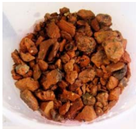
Substrate 1 (crushed brick): the highest drainage ability, but the poorest storage ability
