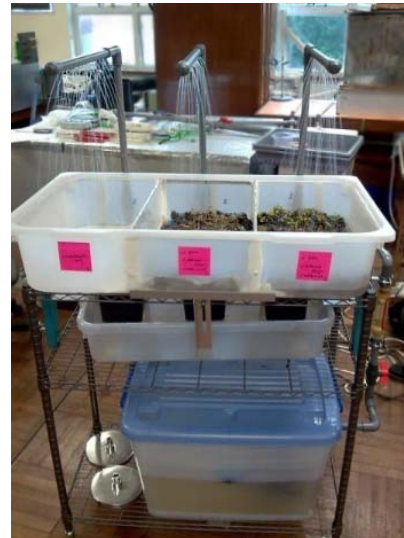
Fig. 6 Experimental set up for testing green roof modules and materials
