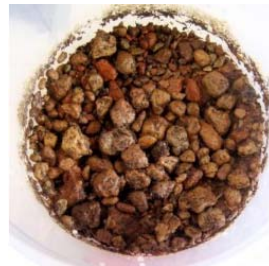
Substrate 3 (crushed stones): high drainage ability, but cannot store water
